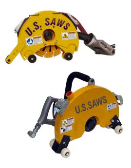
The U.S.SAWS Air Powered Belly Saw is designed to provide a safe alternative to other cutting methods that can be difficult and dangerous because of pipes' subgrade location. The critical factor that gives ease and safer operation is that the tool is strapped to the pipe and is drawn around the pipe, creating a straight and efficient cutting process. Other key factors are that the tools can run in wet conditions without fail because of air or hydraulic power sources.
