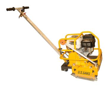
The U.S.SAWS SRX-150 is a compact, lightweight early entry saw designed to cut green concrete to control cracks. The saw is compact and lightweight, the SRX-150 series of dry cutting saws are engineered for early entry sawing of crack control joints within one to two hours of concrete finishing. The blade guard features a vacuum port to control dust when dry cutting.
